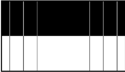
The NEEDLE pattern is symmetrically divided into top half and bottom half. The top half has black background with white vertical needle pulse lines and the bottom half has white background with black vertical needle pulse lines.
